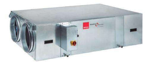
**Heat recovery units** with high-efficiency counterflow Aluminium plate heat exchanger (up to 78%) certified by Eurovent, mounted in a galvanized steel double-walled enclosure with internal thermoacoustic fireproof insulation (A1/M0) made of 25 mm thick mineral wool in models 500 to 2500. Circular inlet and outlet flanges with seals in models 500 to 1800, and rectangular flanges in models 2500. Only available in horizontal version.
